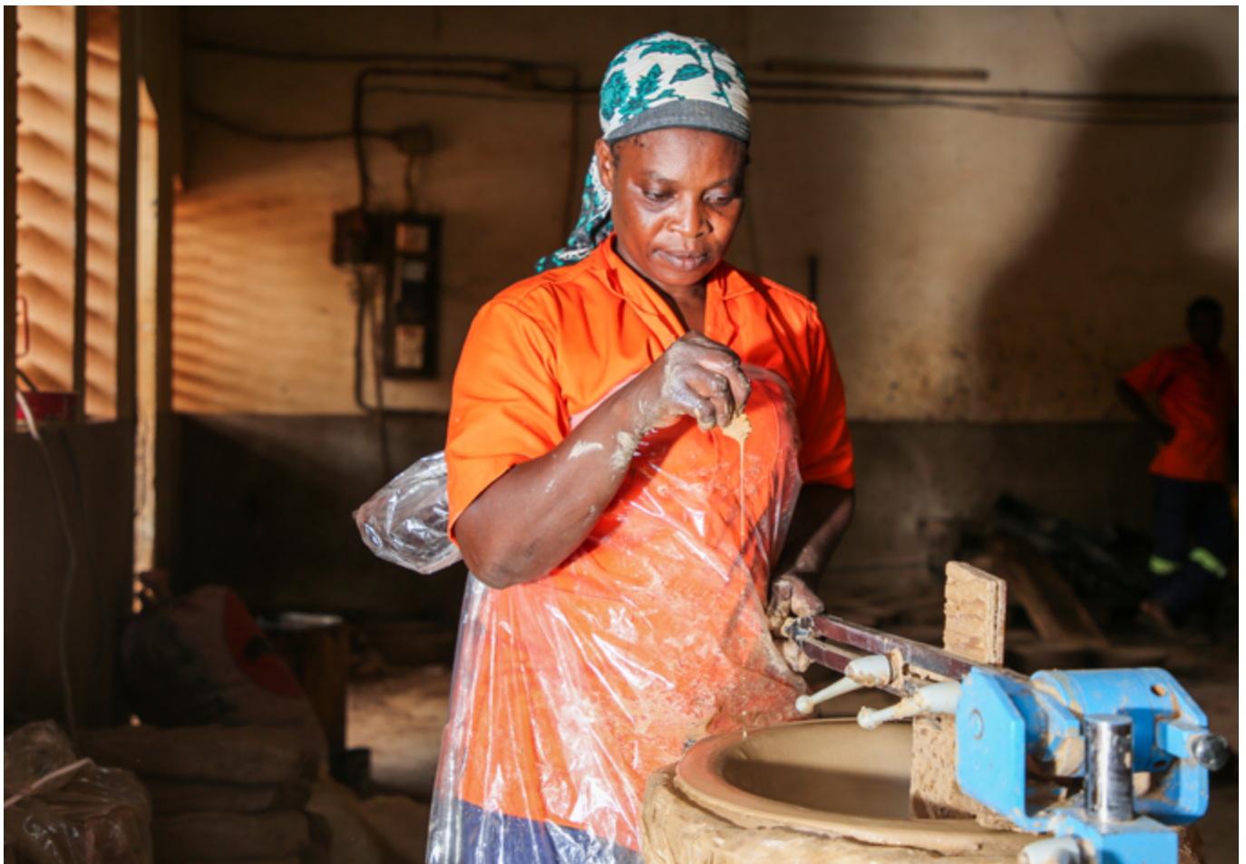
An employee of Porceram, an AECF investee, making a ceramic firebox for an energy saving cook stove in Burkina Faso 1 .
